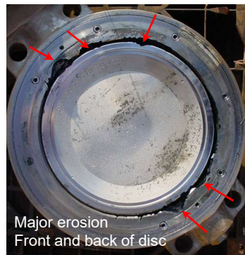
As-received butterfly valve, 4 months in-line
