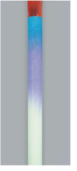
Resin is fully loaded with blue copper
