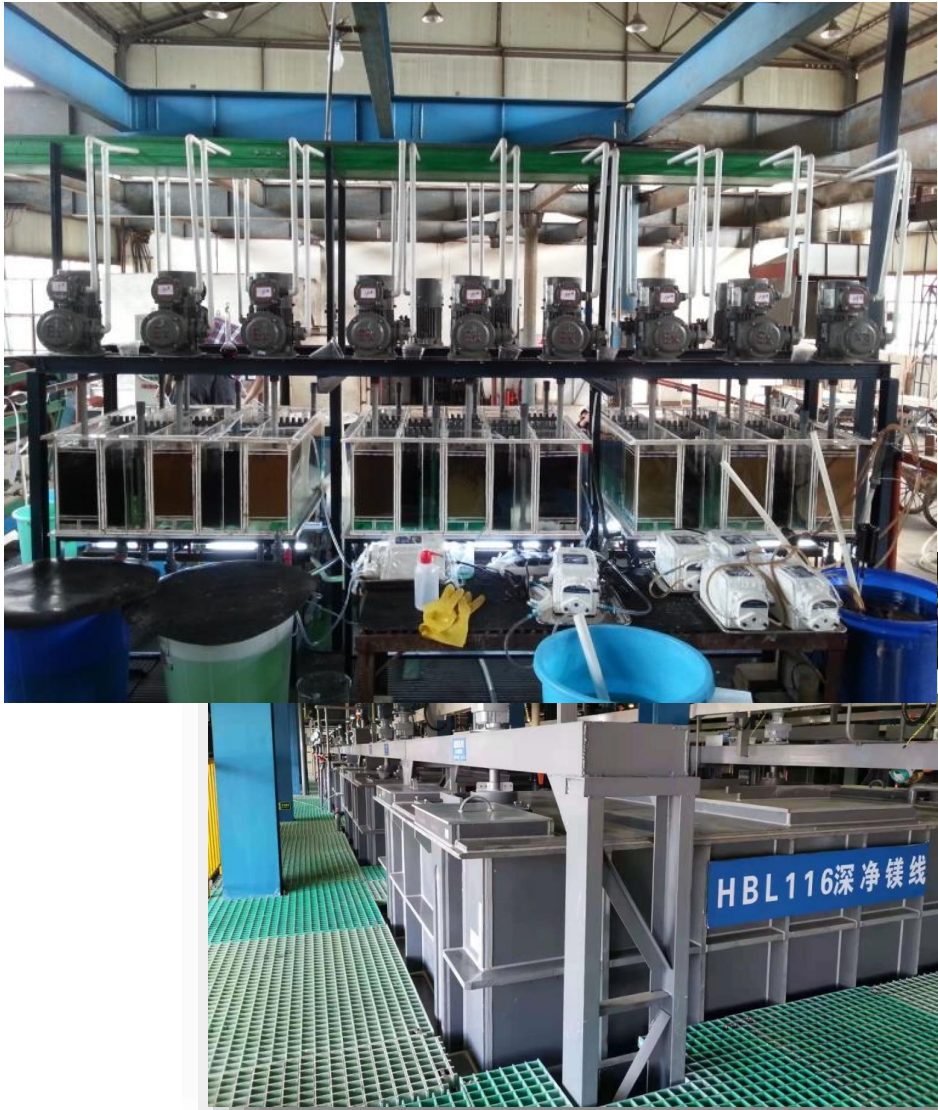
Pilot test & Production Lines: Selectively extraction of Ni/Co from \text{MgSO}_4 solutions by HBL-116(HT-059). Feed solution treating Scale: 400m 3 /day (launched in June 2020 )
