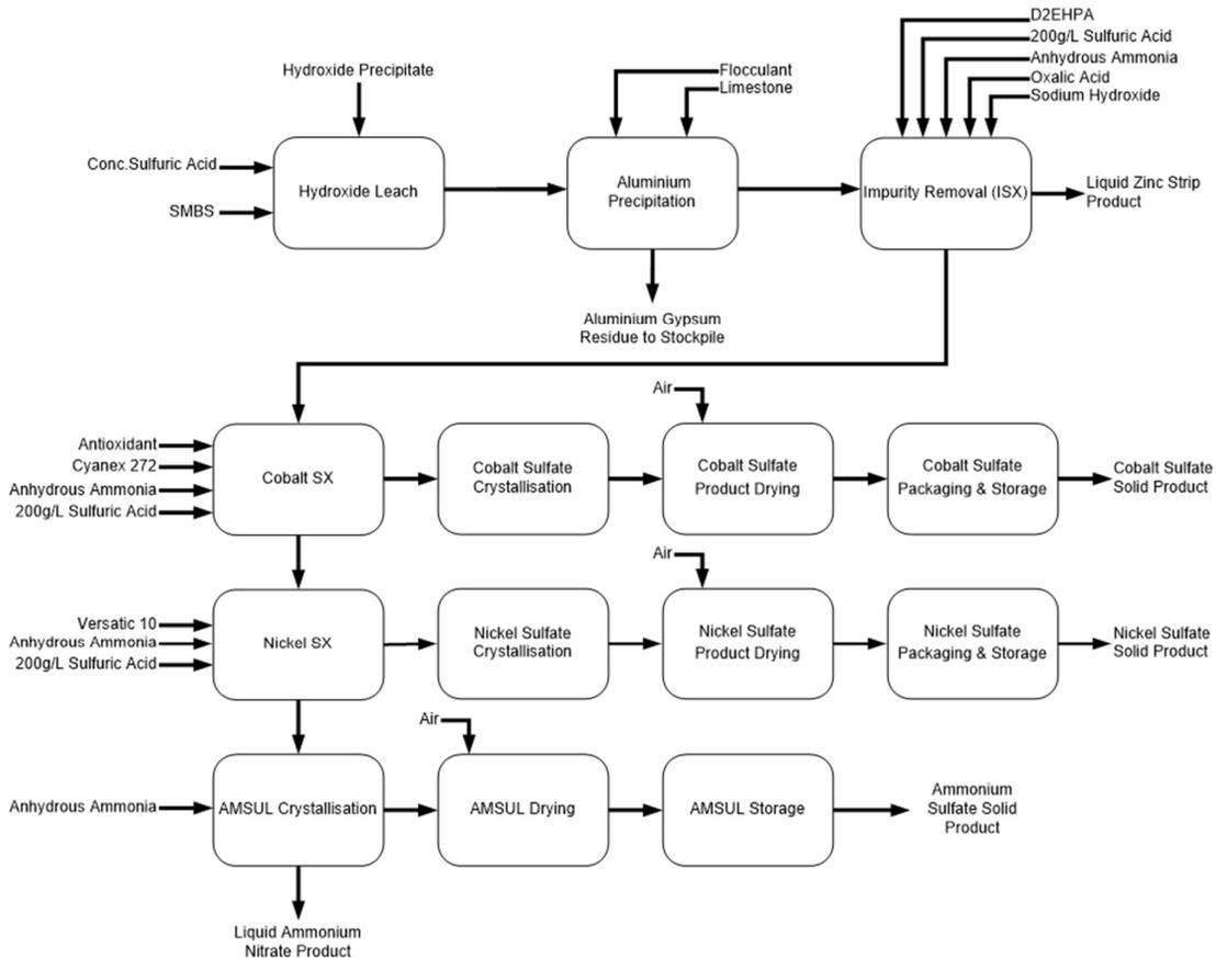
**Figure 1: Simplified Sulfate Refinery Block Flow Diagram**
