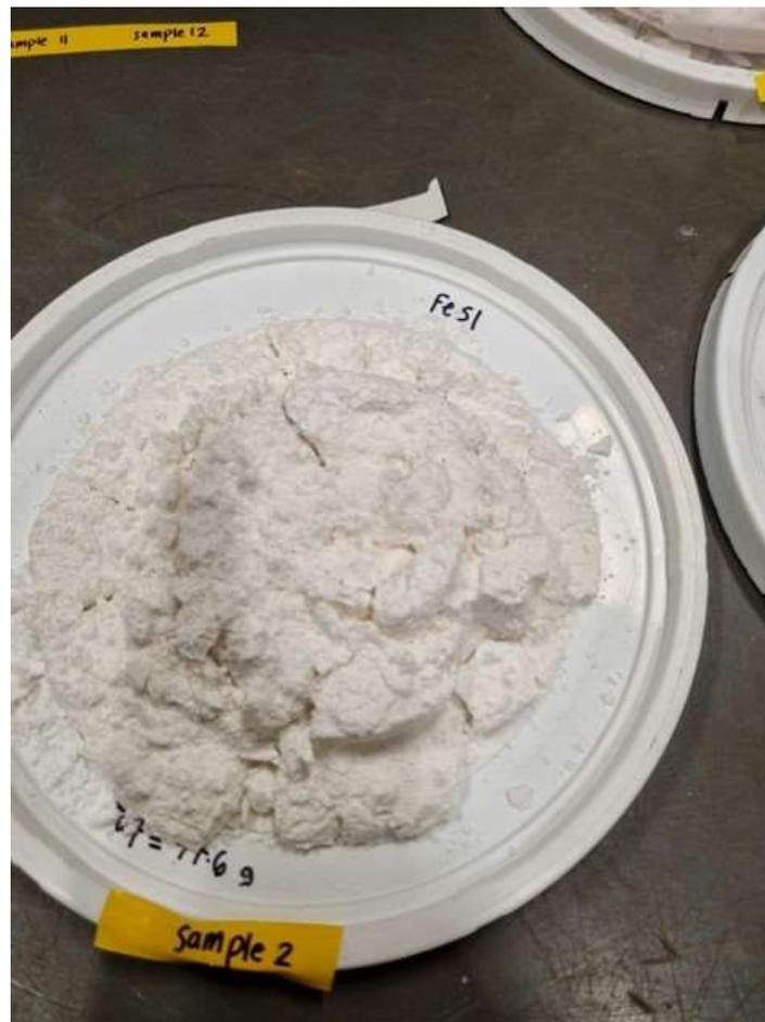
Figure 41: Solids Removed from ISX Fe Strip Settler, May 27
