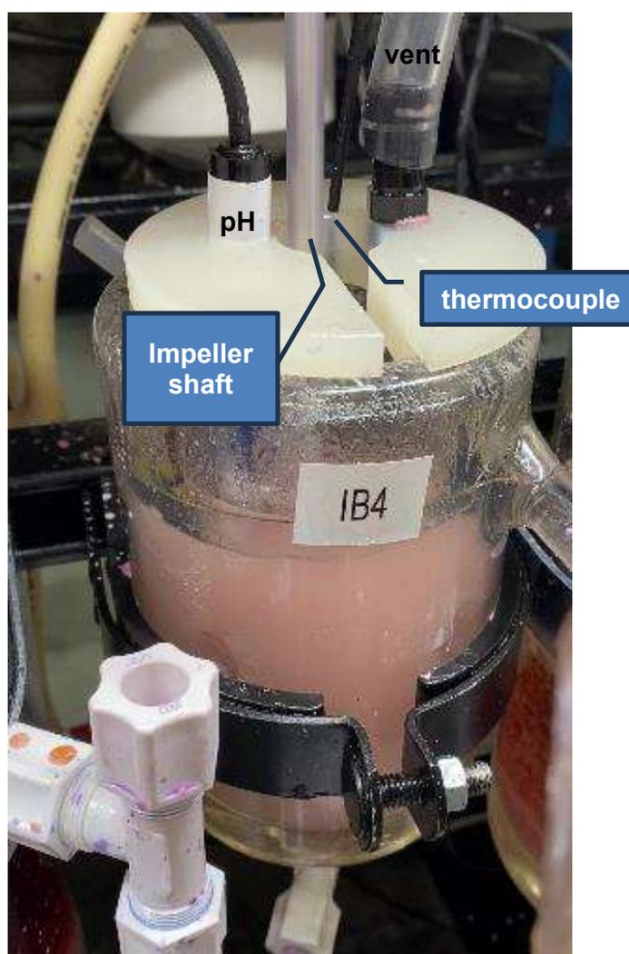
**Figure 7: ISX Scrub 4 Mixer, showing clear plastic vent tubing connected to the slotted cover**
