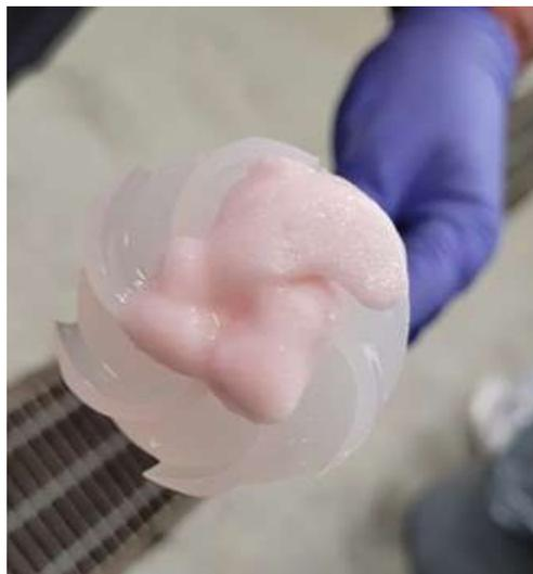
**Figure 35: Gypsum Scaling on ZnIS1 Impeller**
