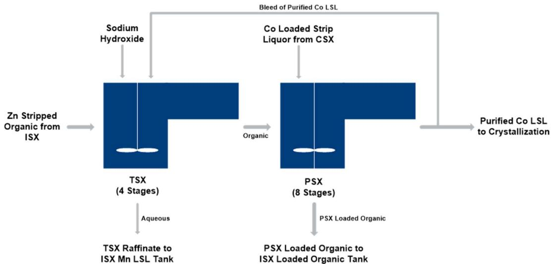
**Figure 4: Schematic of the Proposed Commercial TSX and PSX Circuit**
