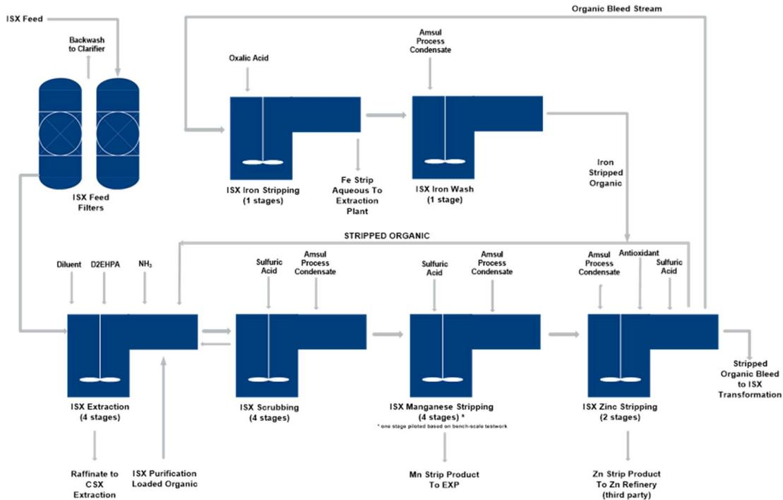
Figure 3: Schematic of the Proposed Commercial ISX Circuit (pre-piloting)
