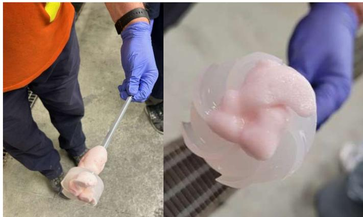
**Figure 31: Gypsum Scale on an ISX Pump-Mix Impeller**
