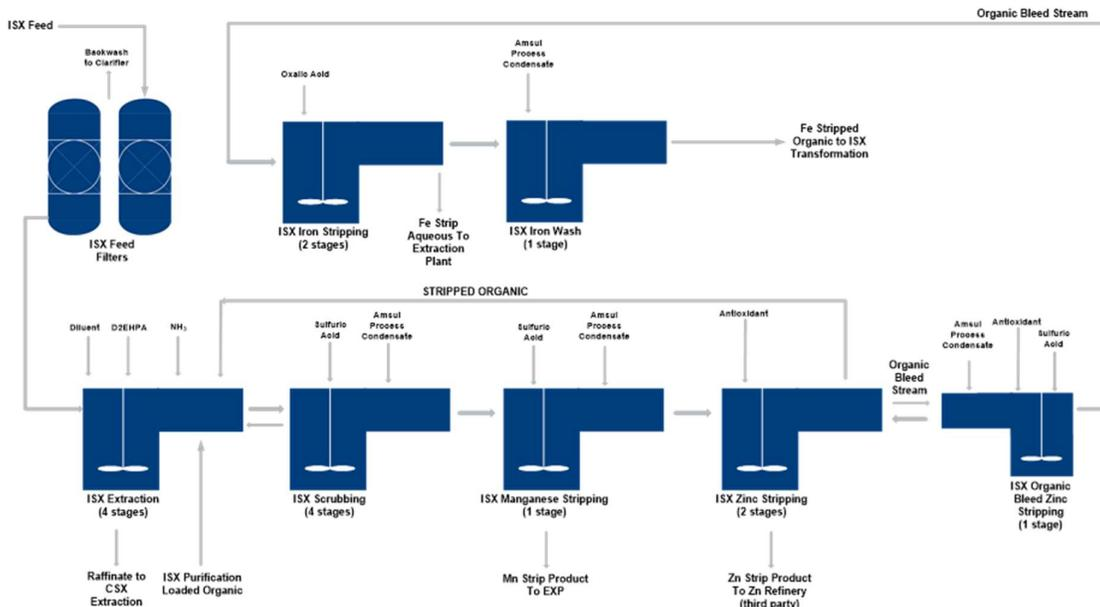
**Figure 51: Schematic of the Proposed Commercial ISX Circuit after Piloting**
