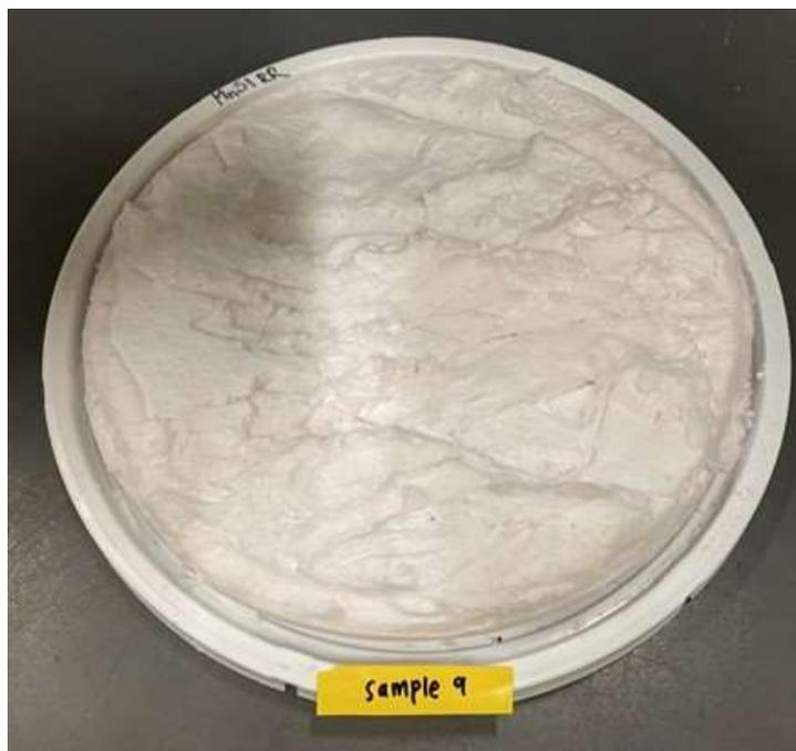
Figure 28: Partially Air-dried ISX Mn Strip Gypsum, May 29
