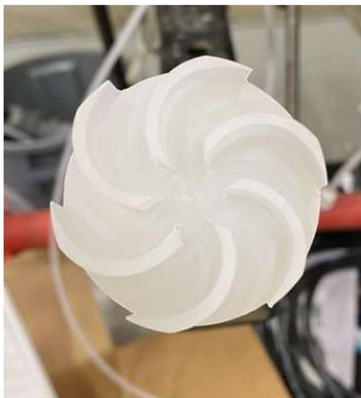
**Figure 6: Photograph of 51 mm Six-Blade Low Shear Pump-Mix Impeller**
