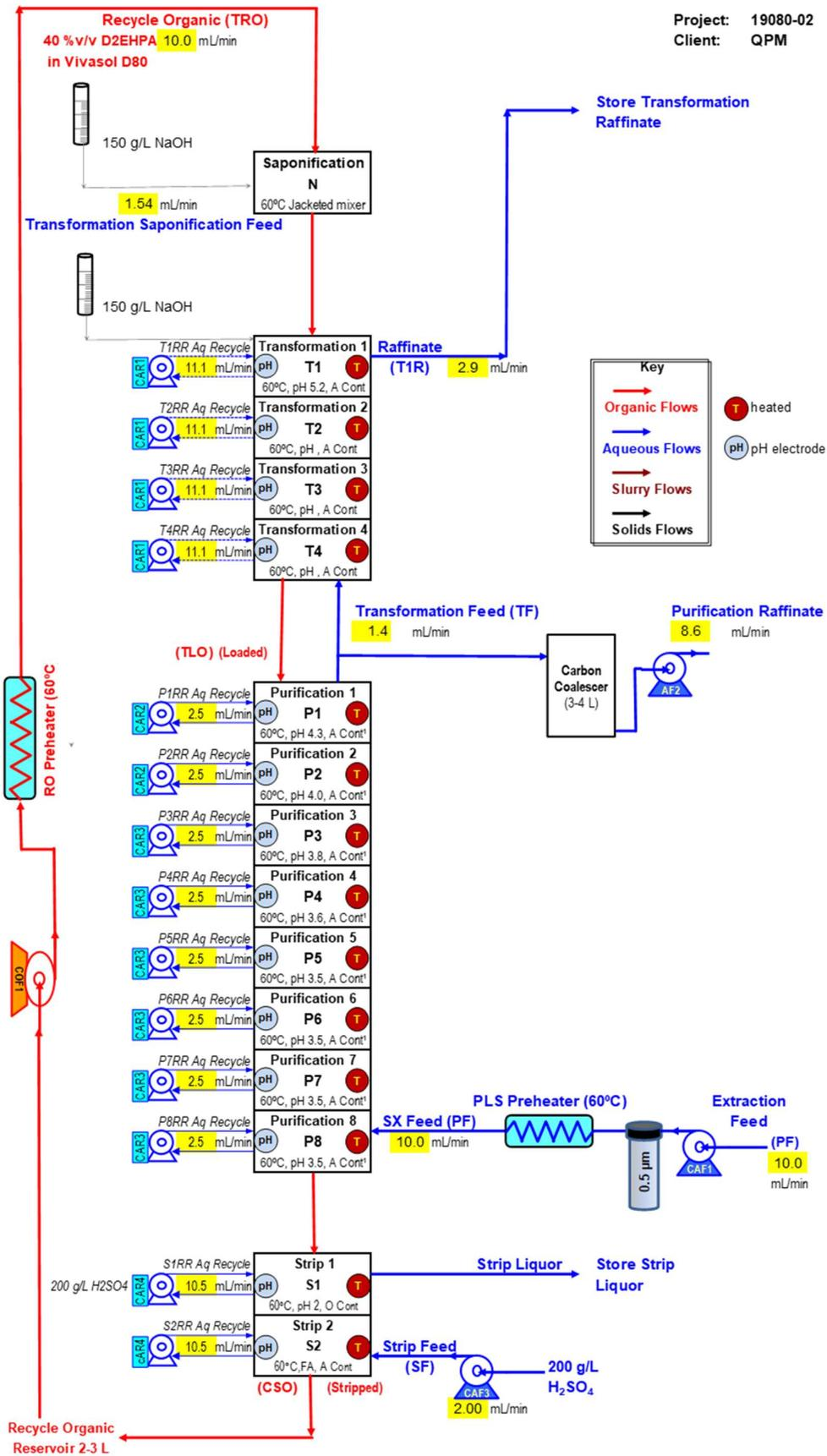
Figure 9: Transformation and Purification Pilot Plant Schematic (source: SGS)
