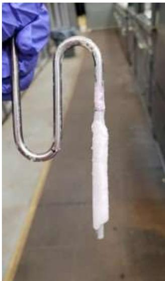
**Figure 32: Gypsum Scaling on 316SS Tube Coupon in Mn Strip**
