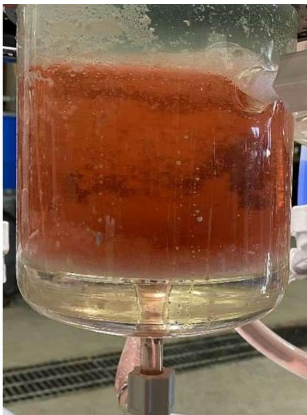
**Figure 19: Gypsum Crud in ISX Scrub 4 Settler**
