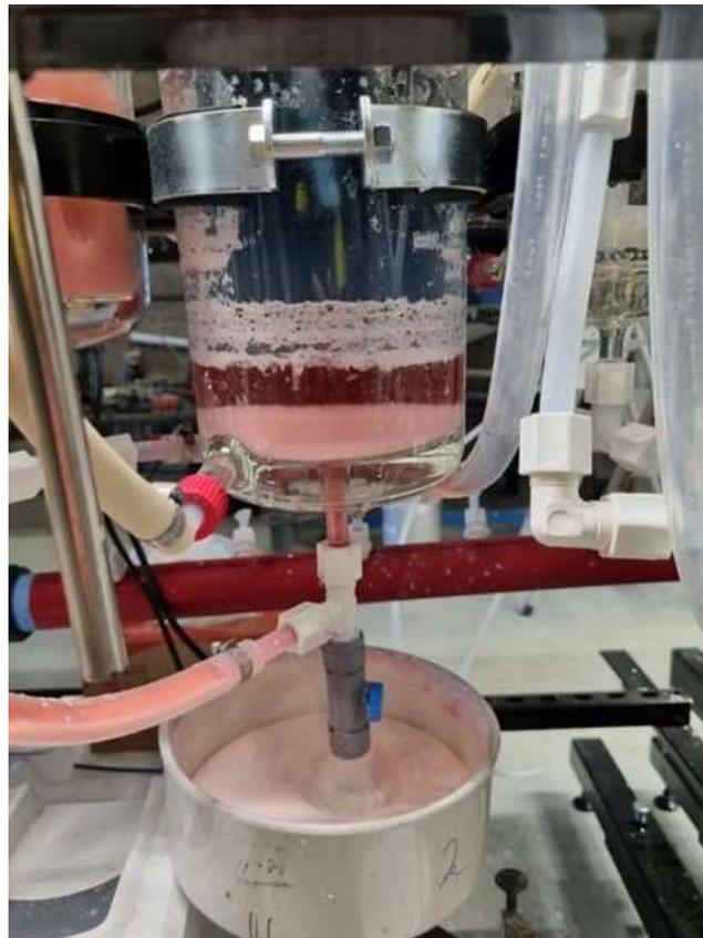
**Figure 27: ISX Mn Strip Gypsum Filter**
