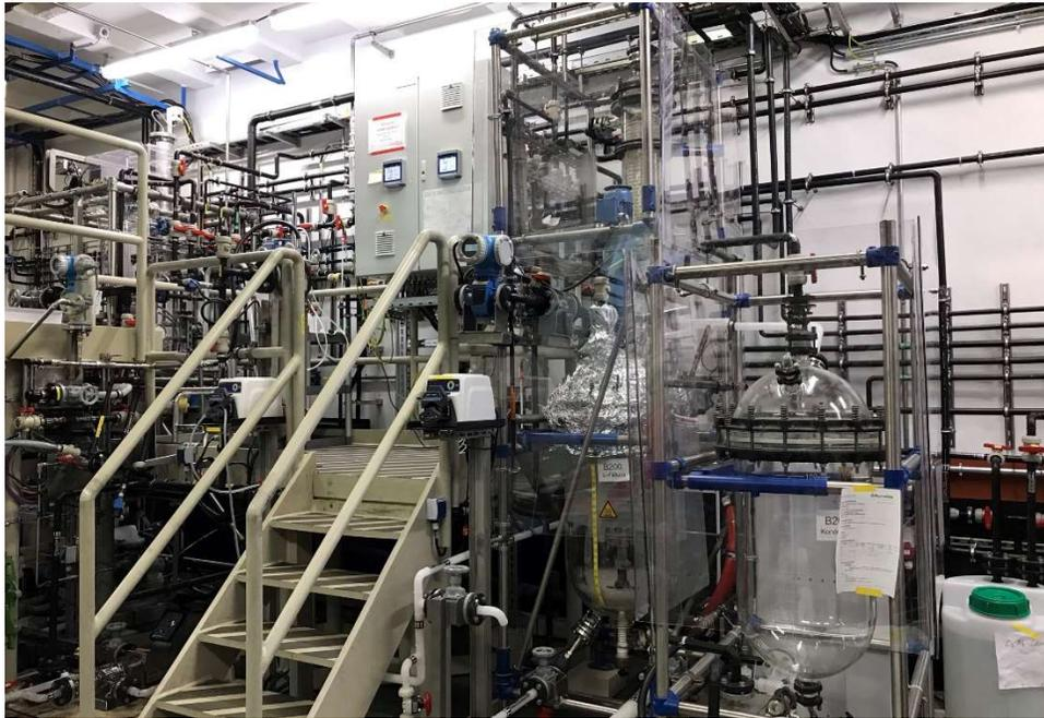
**Figure 3 – Photograph of the Pilot plant showing Reductive leach system and Lithium evaporation system.**
