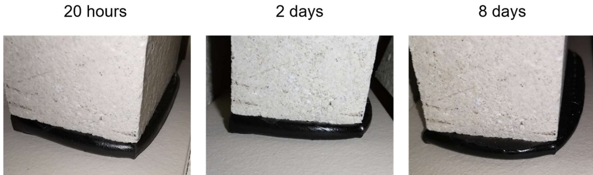
Image 6: Viscoelastic membrane at 80°C (original sheet size: 65 mm x 115 mm, thickness approx. 11 mm) Surface pressure (below a standard ceramic brick 24 x 11.5 x 6.5 cm) \approx 0,052 bar \approx 0,005 MPa After 20 h, 2 days, and 8 days.
