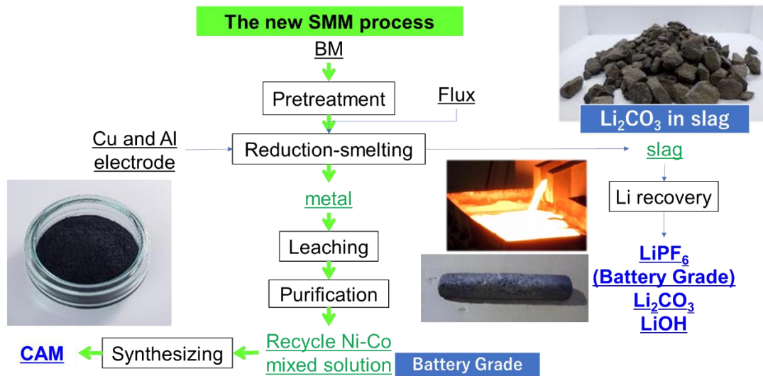
Figure 16. Alloy metal, slag and recycled Ni-Co mixed solution in SMM's pilot plant
