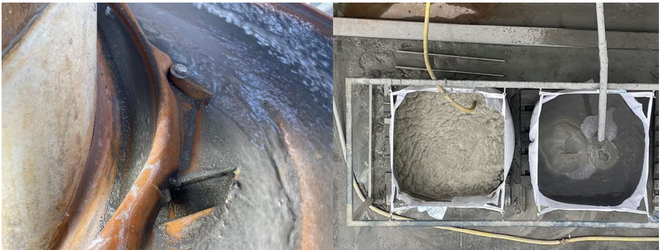
Figure 5: Separation of pyrite on the gravity spiral (LHS), concentrate bags (RHS)
