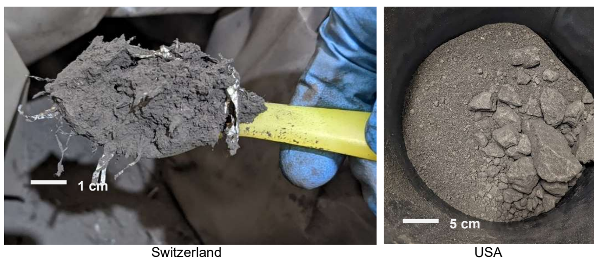
Figure 4: Black mass samples, as received
