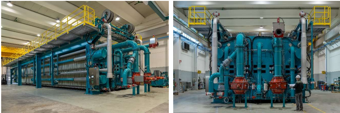
Figure 9: The scale of copper tailings dewatering today requires very large filters such as Diemme Filtration's GHT5000.
