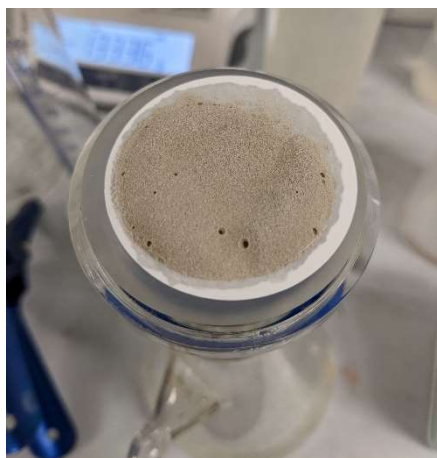
Figure 11: Crude lithium carbonate precipitate from liquor remaining after bulk hydroxide precipitation
