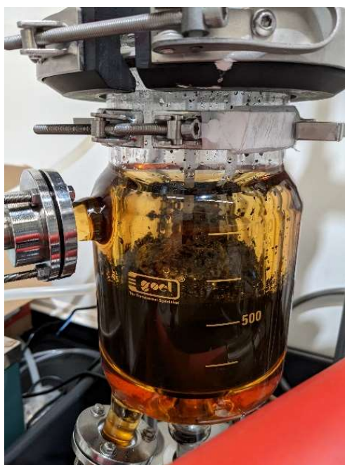
Figure 6: Black mass leaching – note frothing
