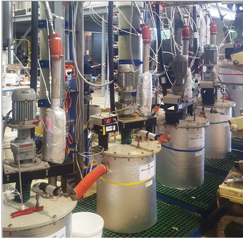
Figure 8: Pilot Co-Current Leaching Circuit
