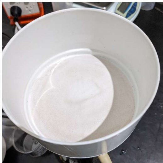
Figure 9: Gypsum residue from neutralisation of free acid in black mass PLS
