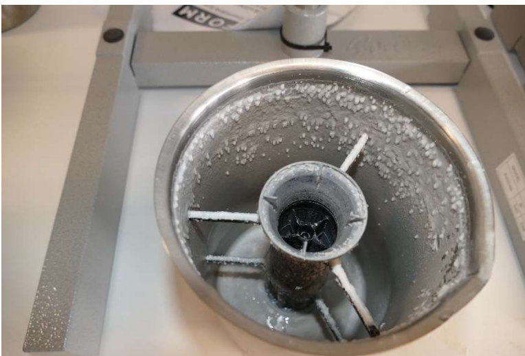
b) Draft tube tank
