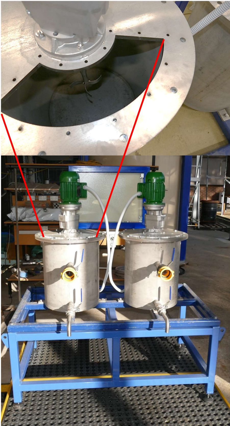
Figure 5: Mixing tank, 50 L, physical modelling to optimise the scale reduction with SWIRLFLOW®
