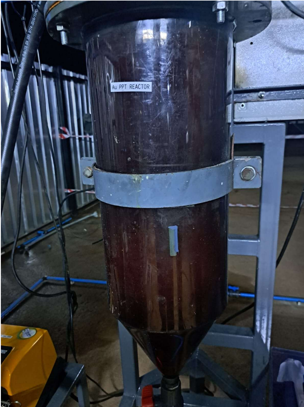
Figure 18: Gold precipitation reactor in action.
