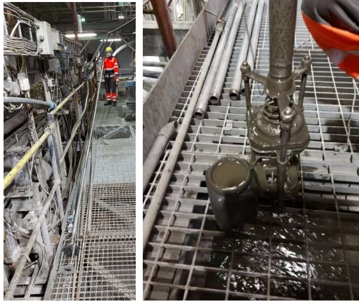
Figure 6. Dip sampler used for the sample collection.
