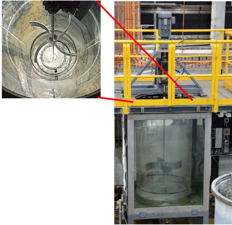
b) Swirl flow mixing tank.
