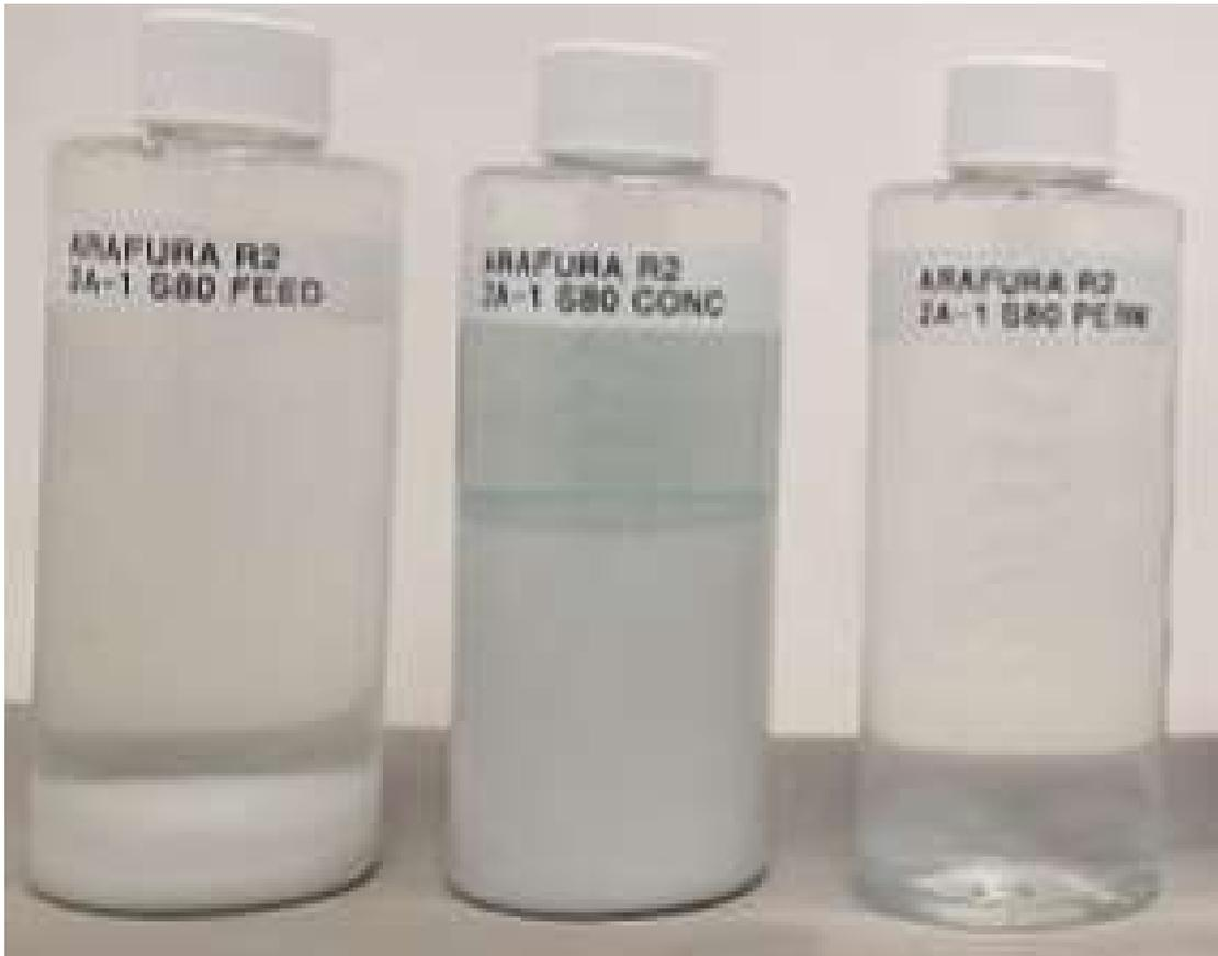
Figure 22 – NF-3 P-Mode NF2A Feed, Concentrate and Permeate (left to right)
