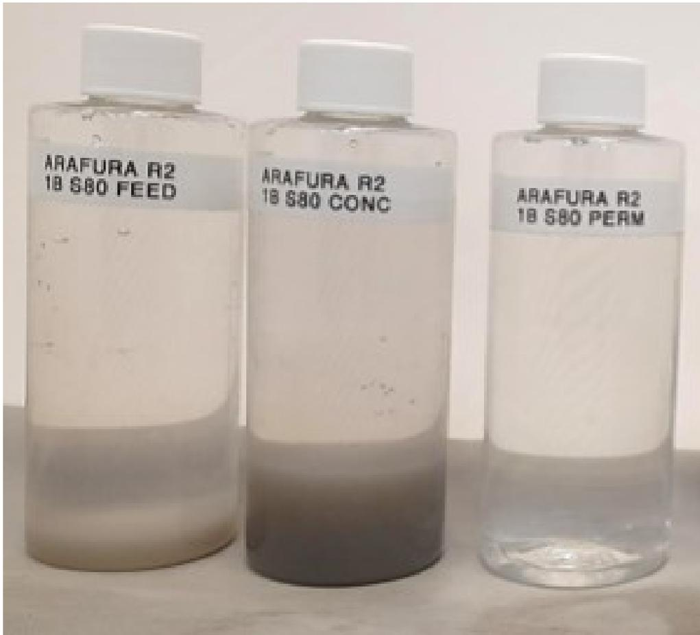
Figure 20 – NF-3 P-Mode NF1B Feed, Concentrate and Permeate (left to right)
