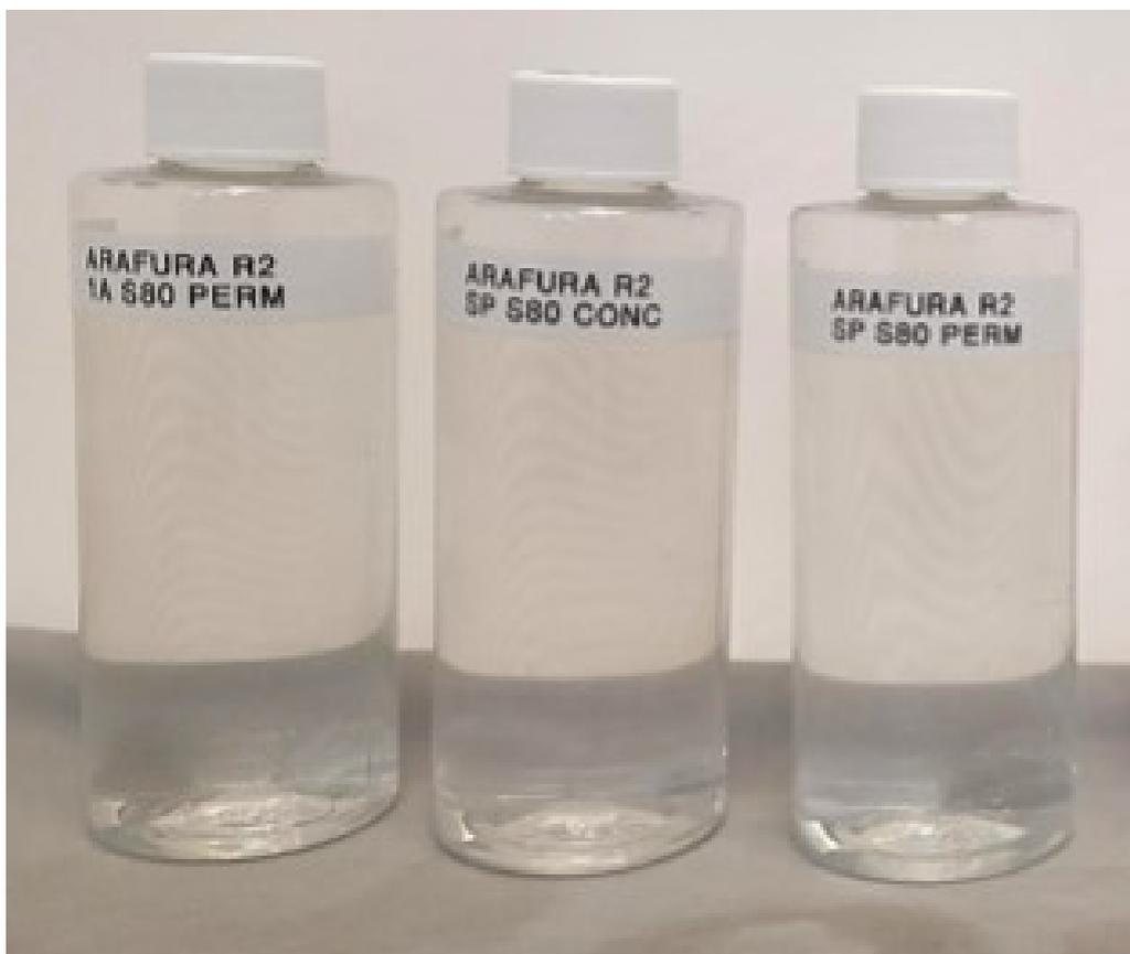
Figure 21 – NF-3 P-Mode NF1 Spiral Feed, Concentrate and Permeate (left to right)
