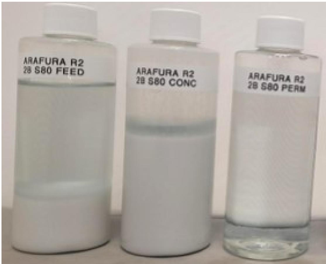
Figure 23 – NF-3 P-Mode NF2B Feed, Concentrate and Permeate (left to right)
