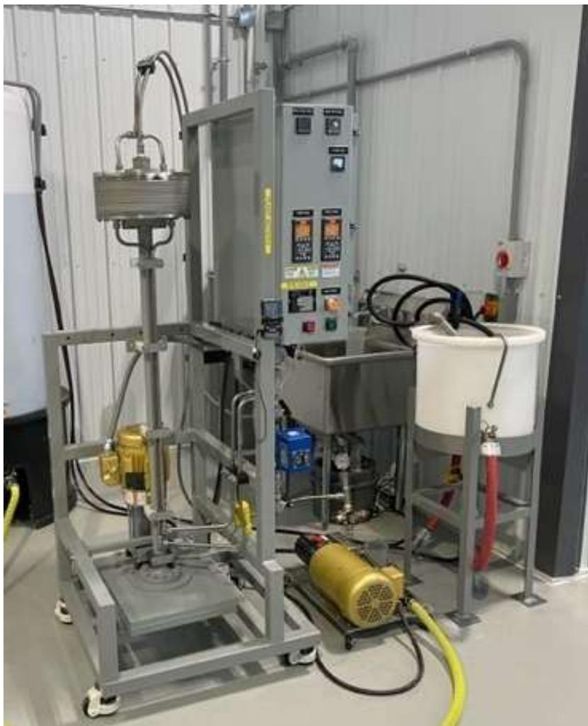
Figure 18 – VSEP LP in P-mode (left) with pump (center) and feed tank (right)
