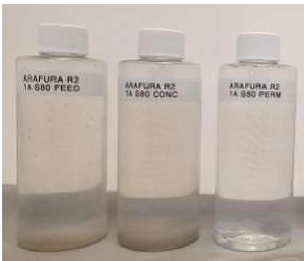
**Figure 19 – NF-3 P-Mode NF1A Feed, Concentrate and Permeate (left to right)**
