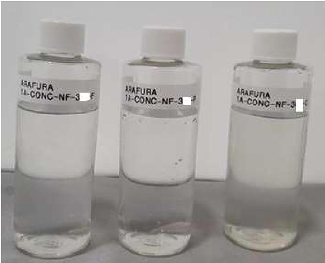
Figure 14 – NF-3 L-Mode NF1A Feed, Permeate, and Concentrate (left to right)
