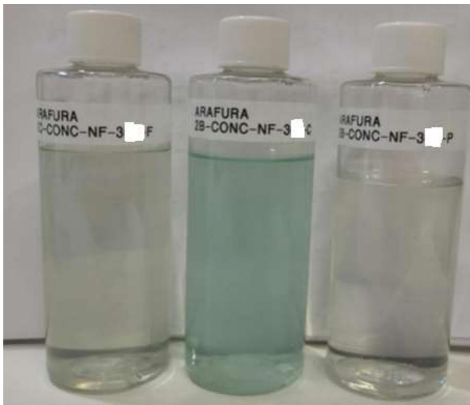
Figure 17 – NF-3 L-Mode NF2B Feed, Concentrate and Permeate (left to right)
