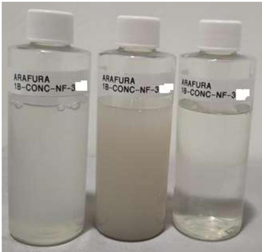
Figure 15 – NF-3 L-Mode NF1B Feed, Concentrate, and Permeate (left to right)
