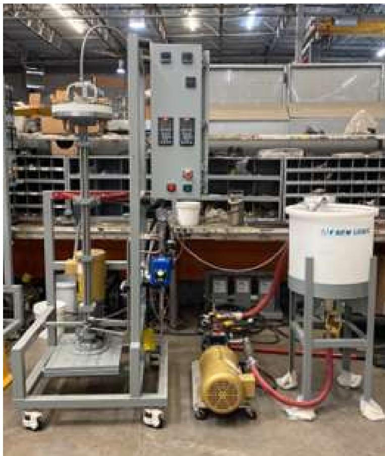
**Figure 8 – VSEP LP in L-mode (left) with pump (center) and feed tank (right).**
