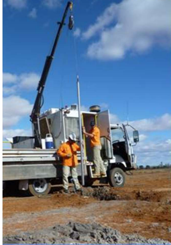
APFN Tool Lowered In To A Drillhole
