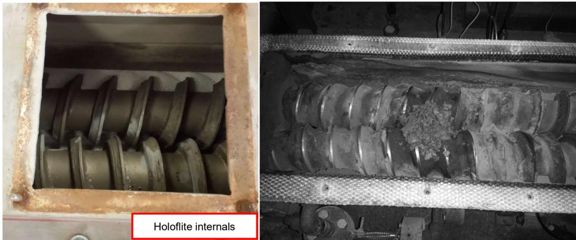
**Figure 9: Pilot Holoflite Internals (Left: before pilot. Right: after pilot)**
