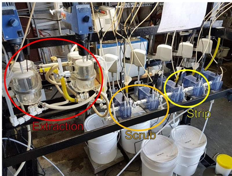
**Figure 14: Solvent Extraction Pilot Apparatus for Th Removal**
