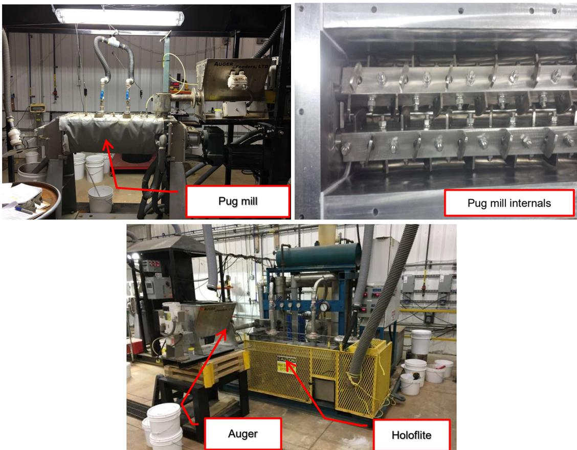
**Figure 8: Acid Feed Mixing and Heating Pilot Equipment**
