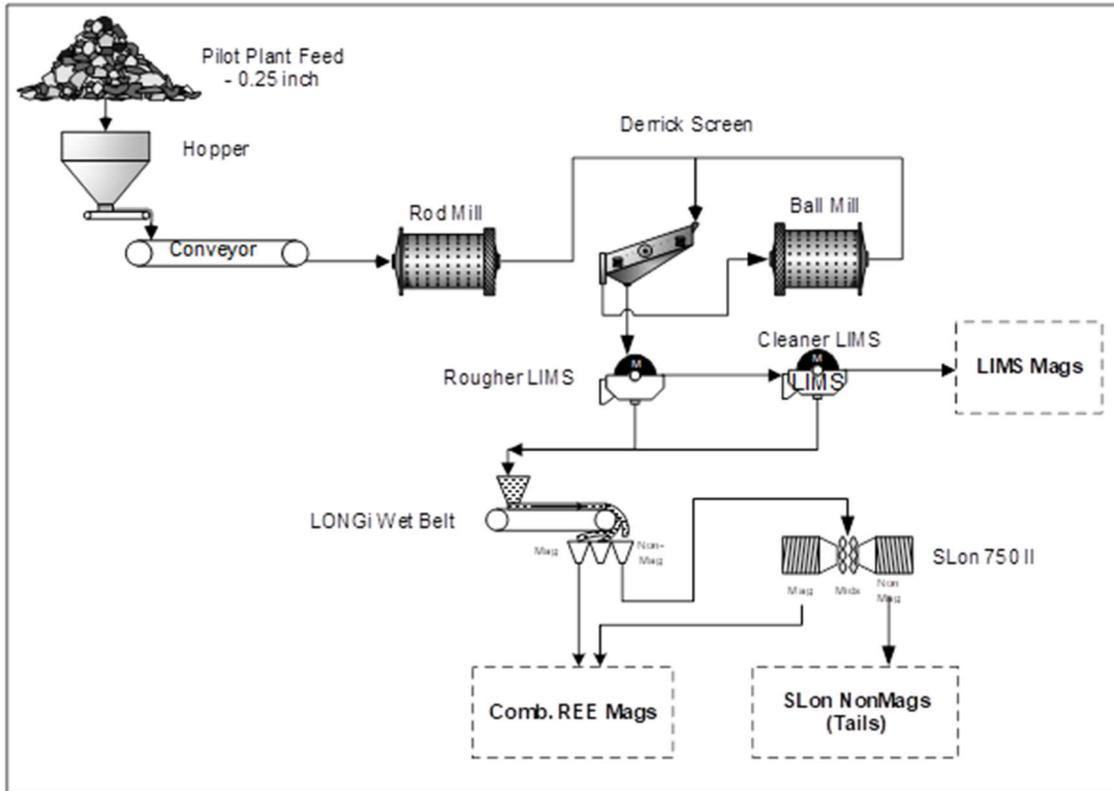
Figure 15: Magnetic Separation Pilot Plant Simplified Flowsheet
