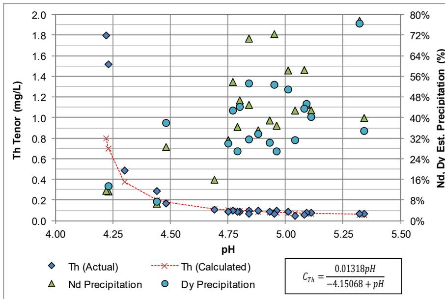
**Figure 11: Relation between Th levels and Nd/Dy Co-precipitation**
