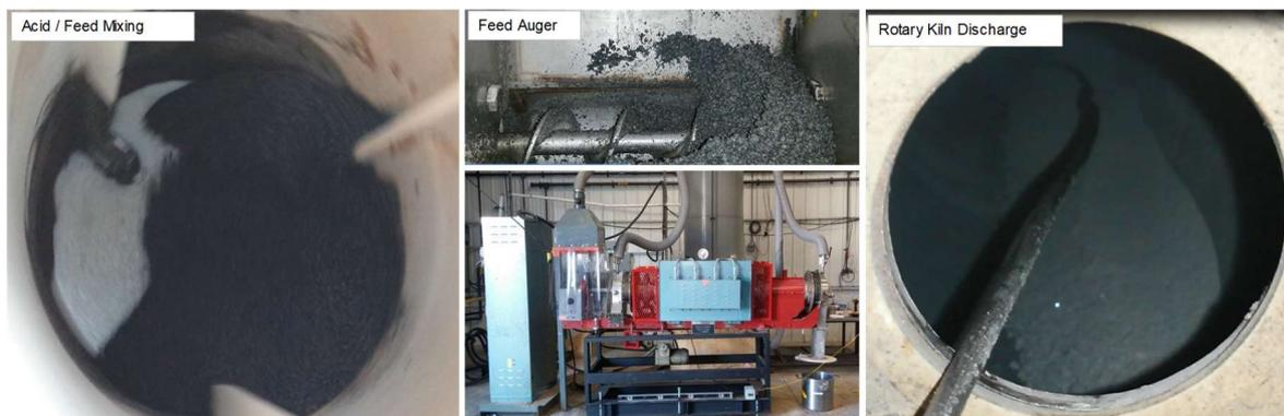
**Figure 5: Acid Bake Operation**
