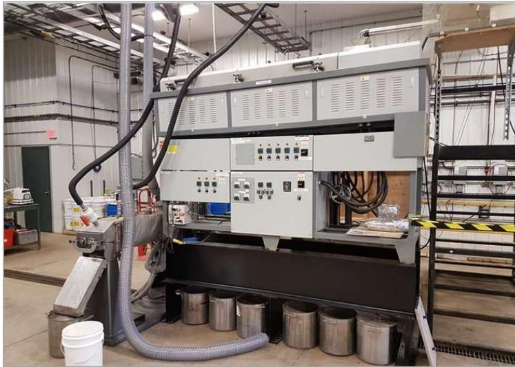
**Figure 12: Screw Feeder and Pug Mill Utilized for Acid/Ore Heat and Mixing**
