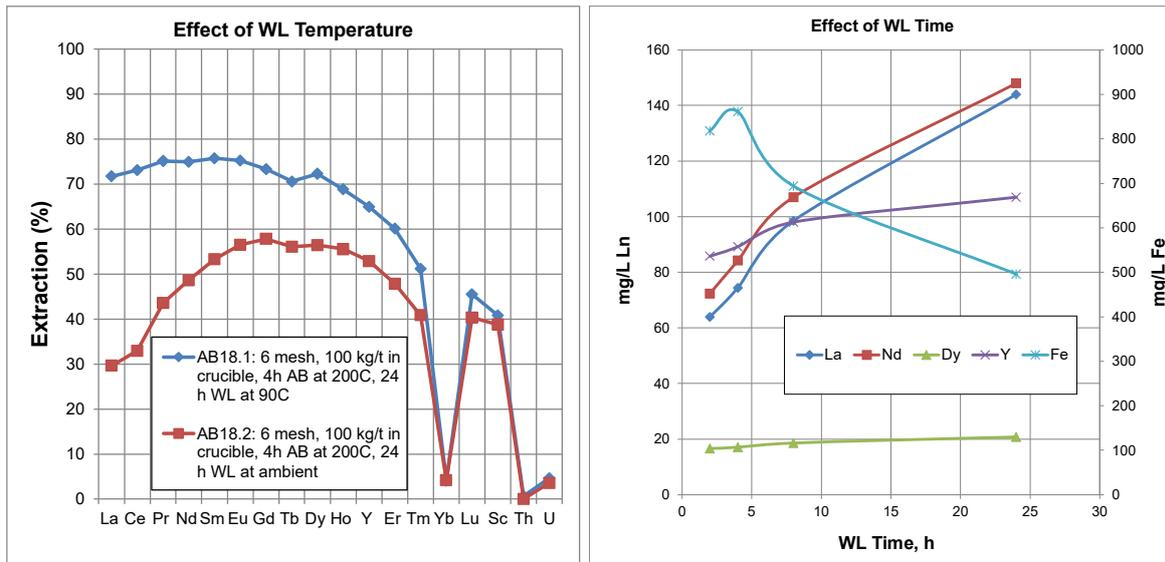
**Figure 4: Acid Bake Testing: Effect of WL Temperature (left) and Retention Time (right)**
