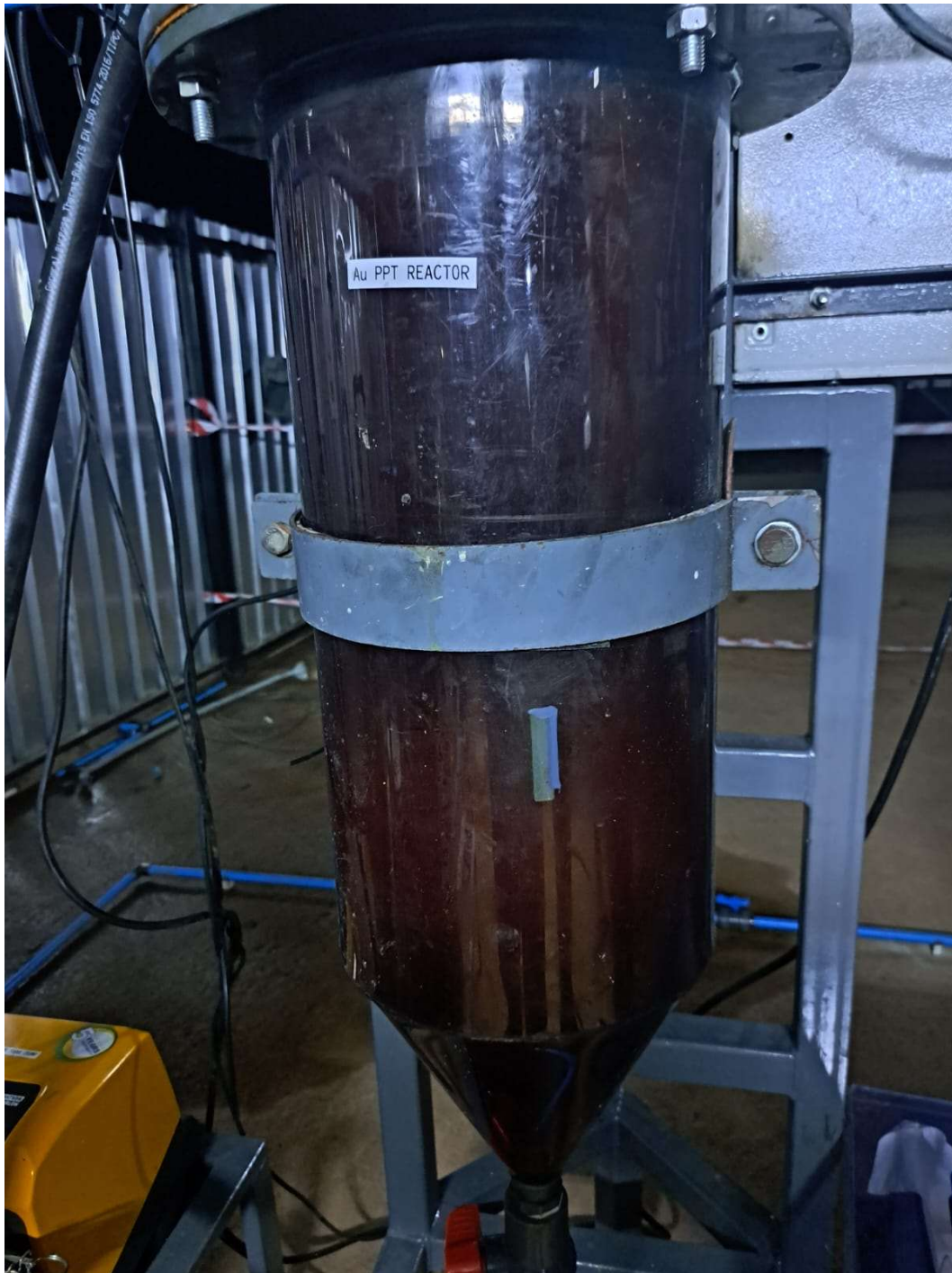
Figure 18: Gold precipitation reactor in action.
