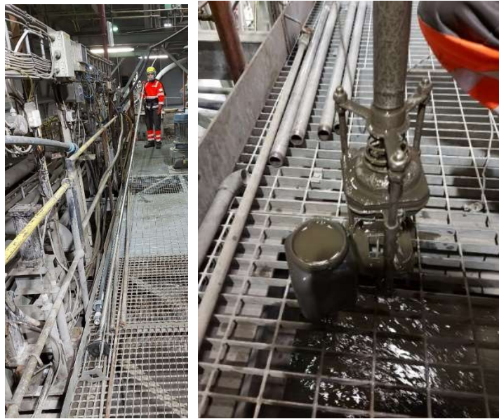
Figure 6. Dip sampler used for the sample collection.
