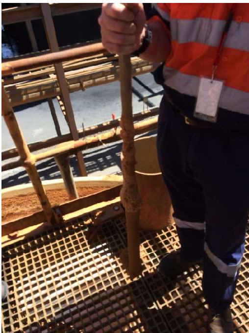
a) Probe/rod that scale grows on
