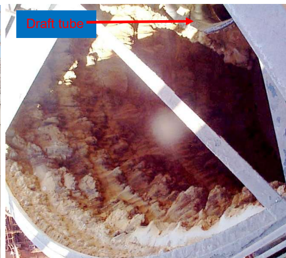
b) Draft tube with scale formed (Before caustic clean)
