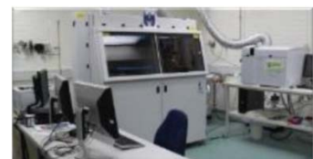
Resonetics S-155-LR 193nm excimer laser ablation system coupled to an Agilent 7700x quadrupole ICPMS.
