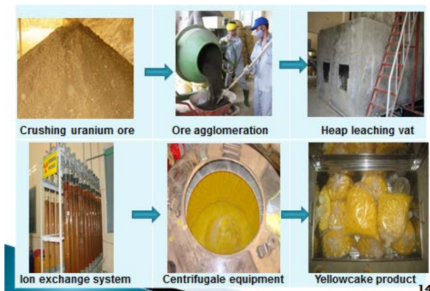
Fig. 8. Heap leaching on pilot scale at uranium deposit in Quang Nam province
