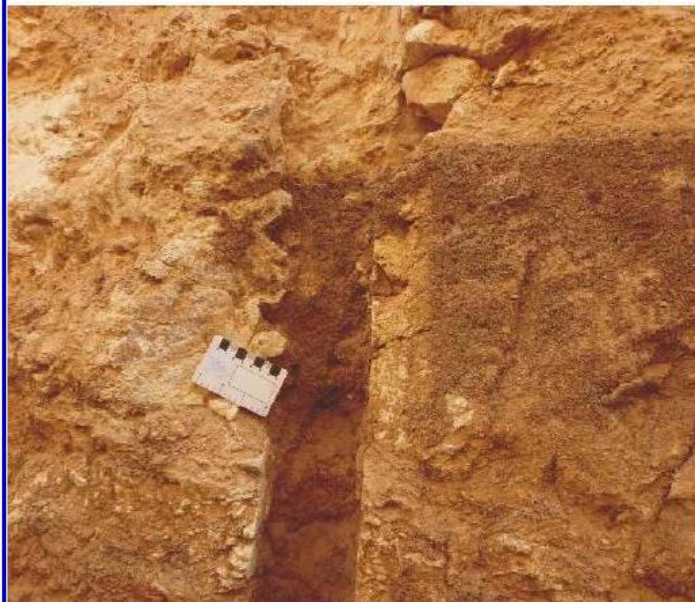
Figure 2: Channel sample cut in the trench wall by a diamond saw (Courtesy of JUMCO)
