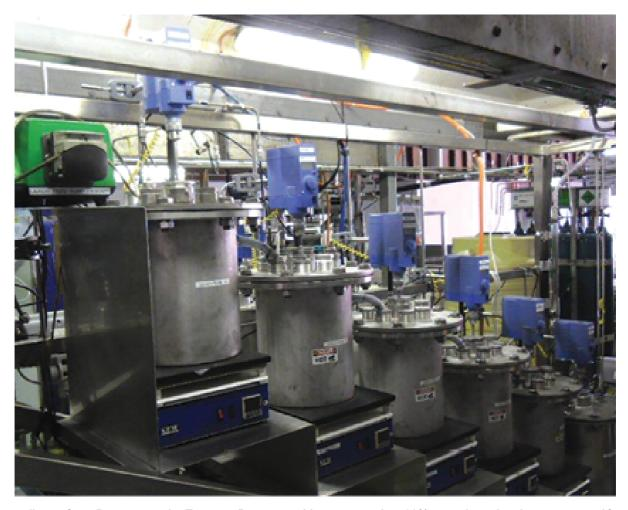
According to Core Resources, the Toowong Process achieves more than 90% arsenic and antimony removal from many copper, lead and nickel concentrates. Process testing has included a pilot plant operation for Tampakan concentrate, successfully reducing arsenic content from 1.1% to 0.1%.
