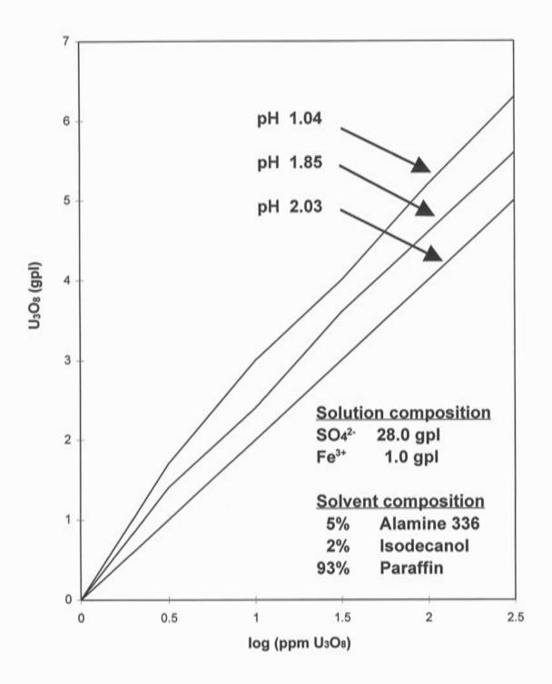
Figure 3. The Effect of pH on the Loading of U<sub>3</sub>O<sub>8</sub> on Tertiary Amine Solvent
