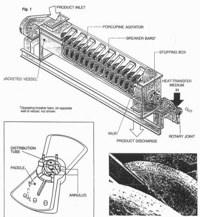
Fig. 2 Paddle cutaway indicates flow of heat-transfer medium from paddle to paddle.
