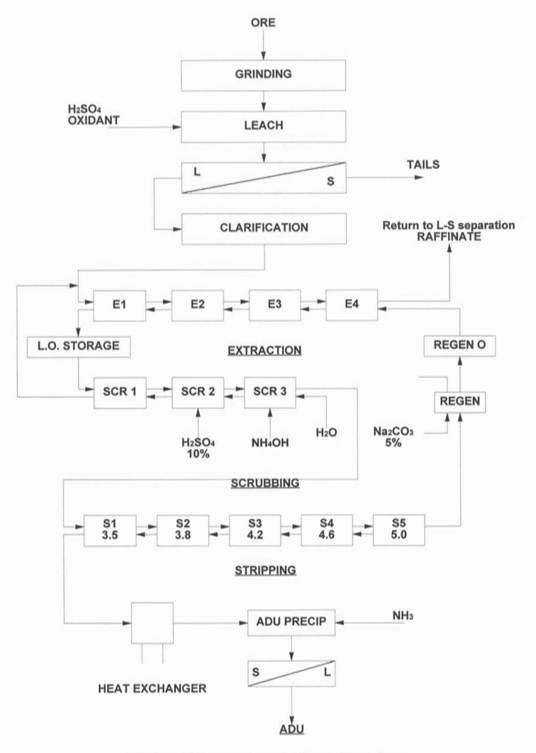
Figure 5. Typical Acid Leach - SX Uranium Circuit ALTA Free Library www.altamet.com.au
