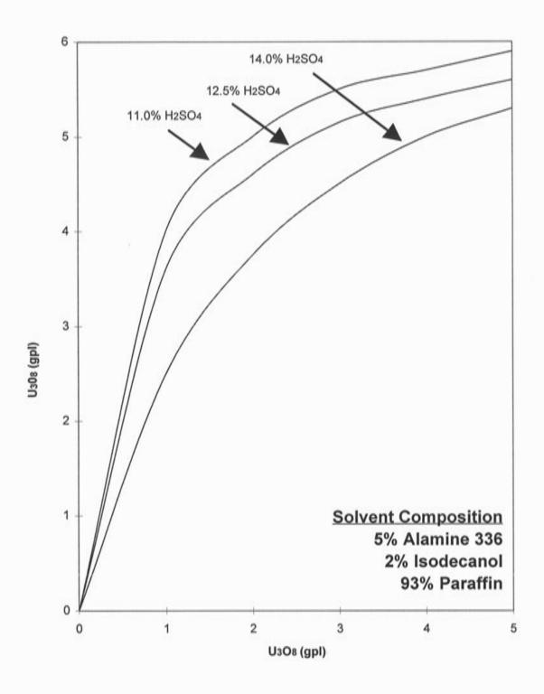
Figure 4. The Extraction of U3O8 from H2SO4 Solution
