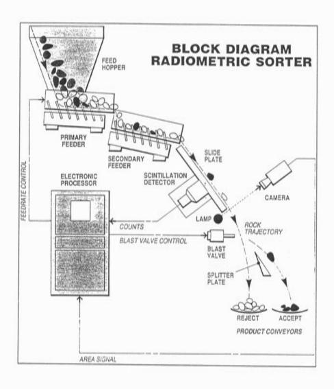
Fig 5 Yeelime Uranium Simplified Block Process Fowsheet
