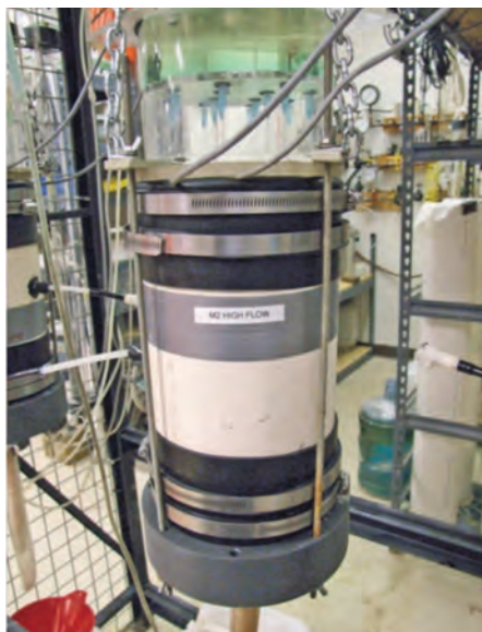
Flexible wall unsaturated flow apparatus as recommended by GeoSystems Analysis
