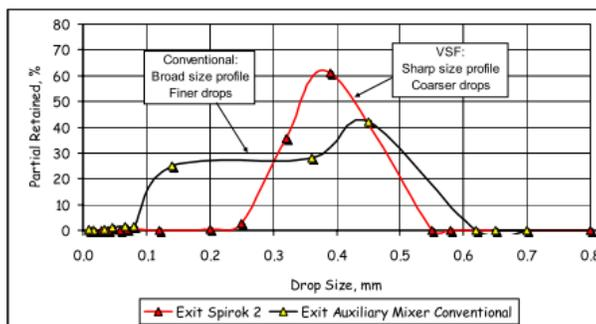
Figure 1: Dispersion Droplet Size Distribution after Mixing<sup>(4)</sup>
