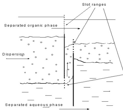
**Figure 3: DDG Fence Operation (Side View)**
