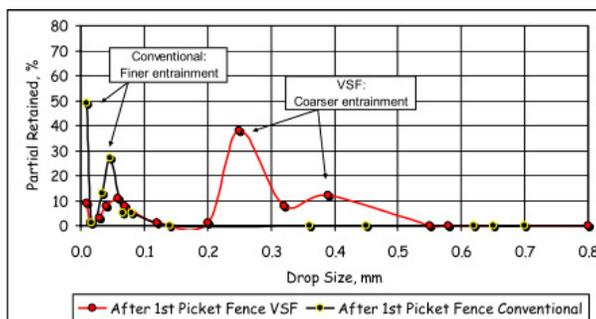
Figure 2: Dispersion Droplet Size Distribution after First Coalescing Fence<sup>(4)</sup>
