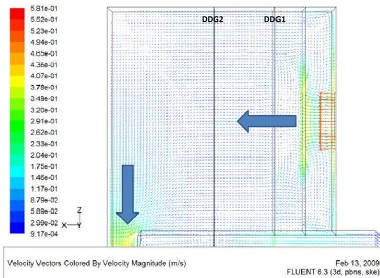
**Figure 4: CFD Model Velocity Profile for Outotec® Reverse Settler Feed Side with DDG Fences**
