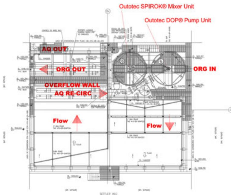
Figure 6: Franke Washing Loaded Organic tank General Arrangement Drawing
