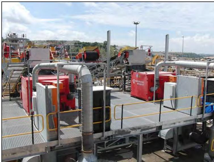
**Figure 16: Kloof plant showing two parallel optical sorters (third sorter to be installed at later stage)**
