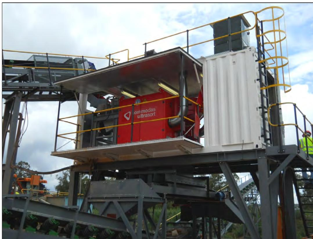
**Figure 21: CommodasUltrason containerised PRO Secondary COLOR sorting plant at CRG**
