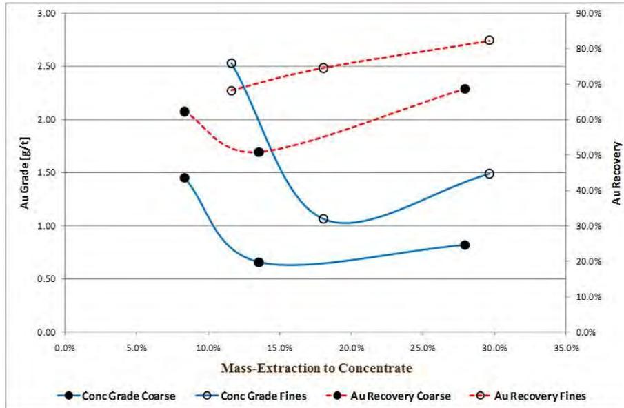
**Figure 13: Au grade and recovery vs. mass-extraction**
