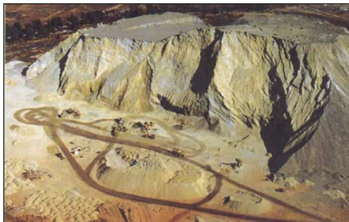
Figure 6: Typical SRD screening operation using mobile screening equipment
