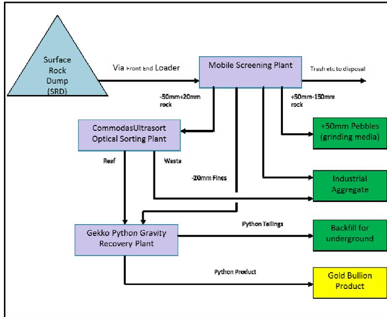
Figure 14: Flow diagram for SRD treatment<sup>(9)</sup>
