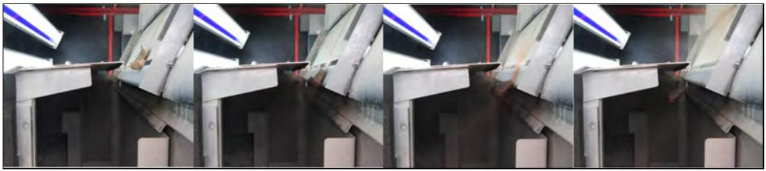
**Figure 2: Picture sequence showing optical detection and ejection of gold-bearing Witwatersrand ore**
