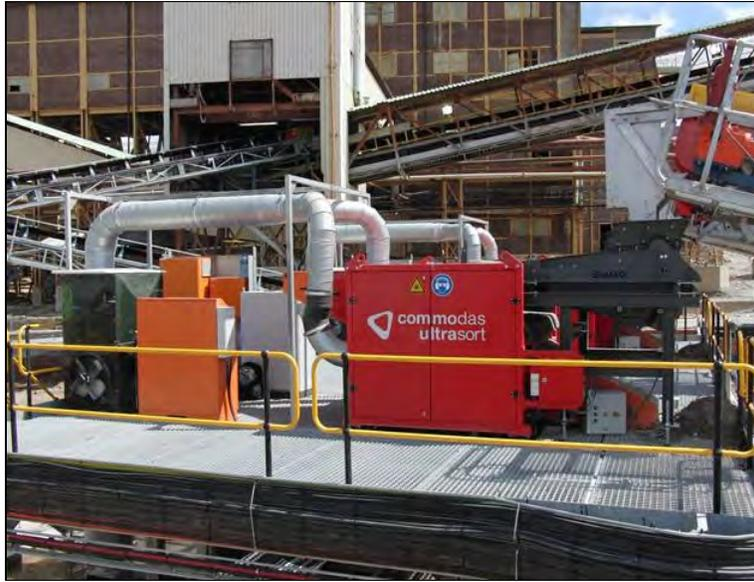
**Figure 15: Installed optical sorter showing feed arrangement, dust extraction and chiller**
