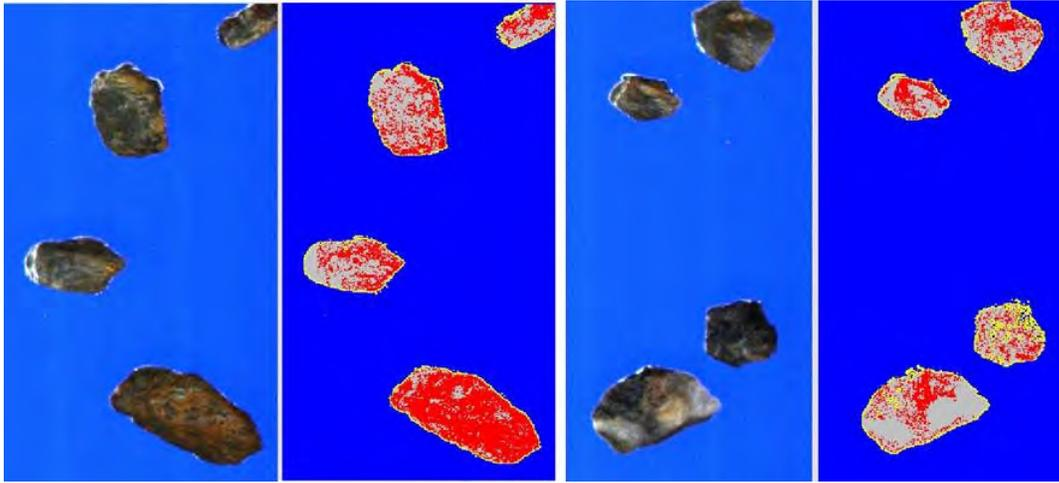
Figure 10: Scanned images of dark reef (left) and light reef (right)
