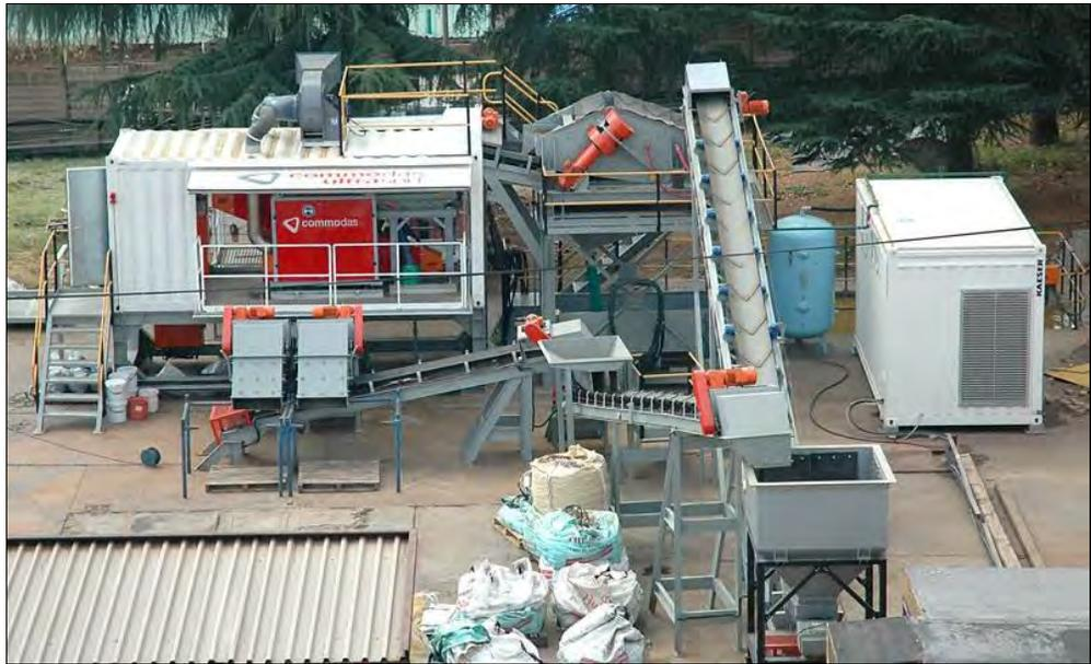
**Figure 9: Optical sorting test center at Mintek**
