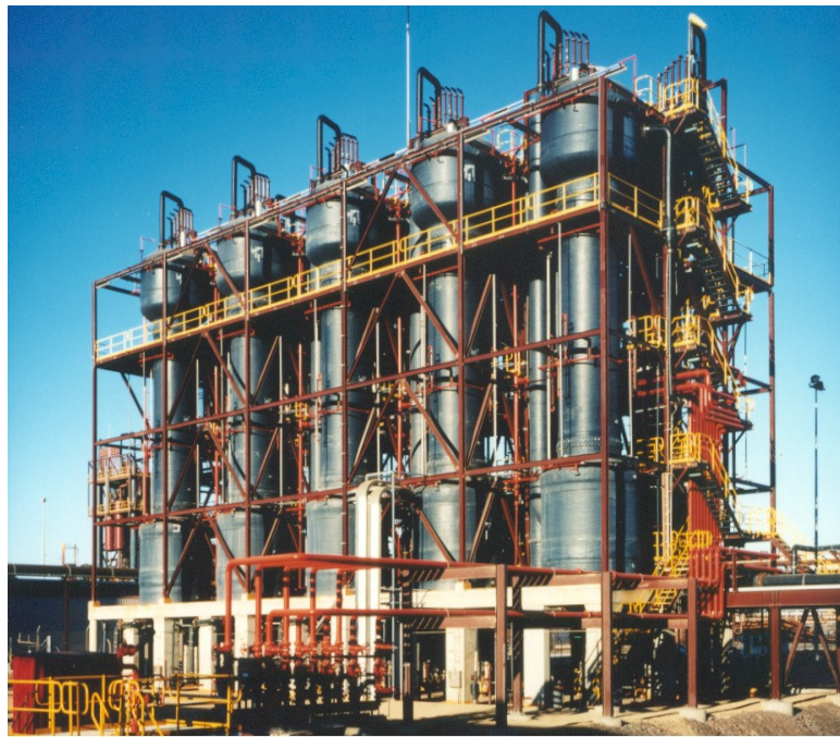
Fig. 6 Bateman Pulsed Column Installation at Olympic Dam
