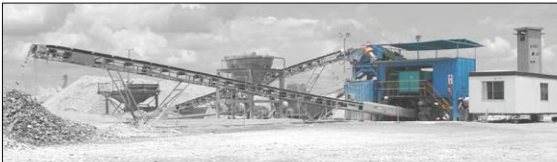
Figure 4: Optical Ore Sorter Pilot Plant at Kloof Gold Mine (Ref. 6 Commodas Ultrasort Paper World Gold 2009)
